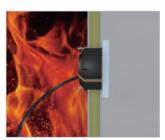
\* In a fire, the volume of HK-200 type class B15 cavity wall box will expand quickly to provide the fire from spreading to different cabins.
