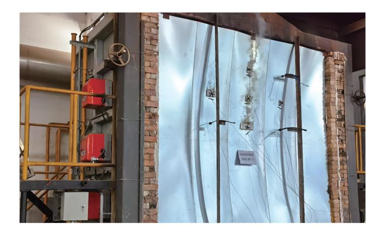
HK-100 type class B15 cable conduits are easily and quickly fitted. It has good firestop sealing performance. In the case of high temperature and fire, the cable conduit will rapidly expand to form a flame-retardant carbon layer, to seal the gap between the bulkhead panel and cable. Therefore, it can effectively prevent the spread of temperature, flames and toxic gases.
